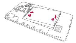
4 To replace the cover onto the device, align the back cover **1** and press it down until it clicks into place **2**.
